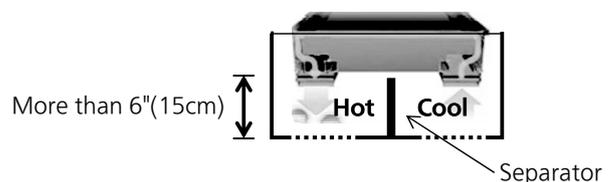
3) When installing the Displays “side by side” or “back to back”, please make sure hot exhaust air is not drawn from the Inlet of the other Display. A separator material may be installed as illustrated.
