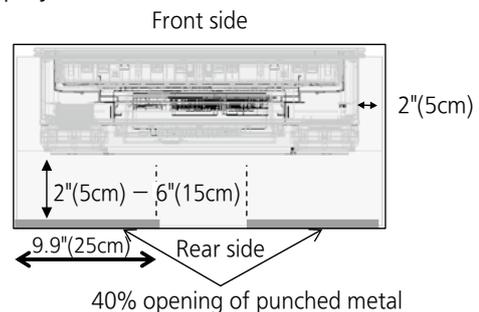
(\*1) When the spacing behind the display exceeds 6"/15cm, exhaust air may not vent smoothly and be drawn into the Display Inlet. To prevent such a situation, a separator material to isolate the intake and exhaust air shall be installed as illustrated.
