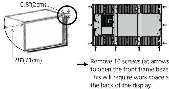
(\*3) The front frame bezel is hinged to the cabinet. 0.8"/2cm of space is required for opening it as illustrated.
